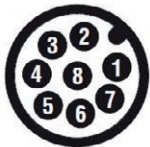
(Connector) M12x1; 8-pole, A-coded
