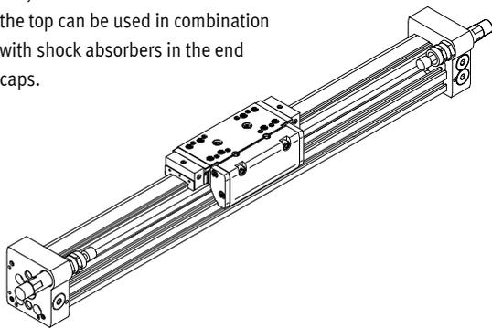
Only the connection on the front or top can be used in combination with shock absorber retainer DADP.
