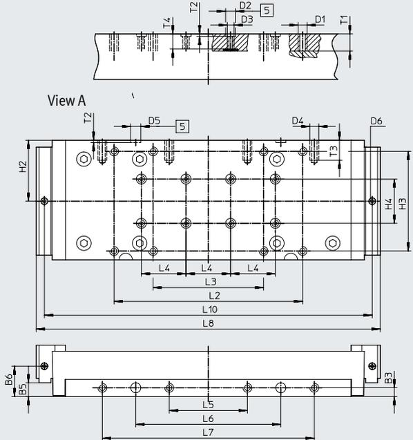
[5] Drilled hole for centring sleeve ZBH
