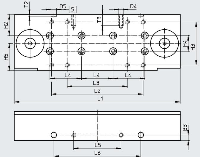
[5] Drilled hole for centring sleeve ZBH
