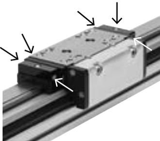
The lubrication adapters enable the guide of the linear drive DGC-KF to be permanently lubricated in applications in humid or wet ambient conditions using semi or fully automatic relubrication devices.
