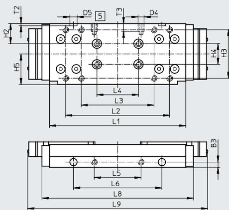
[5] Drilled hole for centring sleeve ZBH
