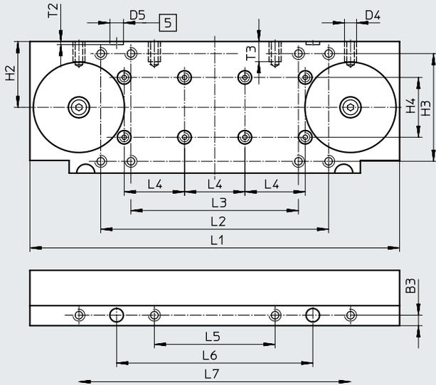
[5] Drilled hole for centring sleeve ZBH
