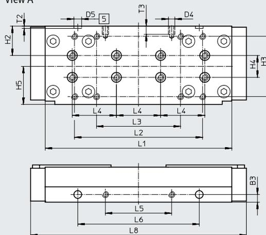
[5] Drilled hole for centring sleeve ZBH
